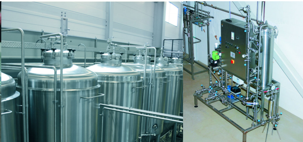
The six fermenting tanks can also be supplied with wort from the two large brewing streams. Alongside on the right a small filter unit with candle filter.
